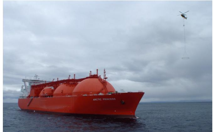
Independent of crew aboard the casualty, the ShipArrestor can be used even if the ship is abandoned. Once the connection is made, the system is fully autonomous.
