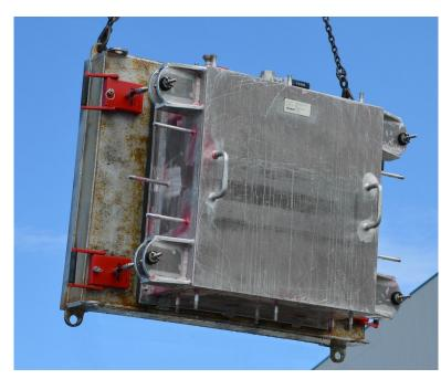
Once the inside has been pumped dry, the pressure difference will compress the rubber gasket further. At this point, the watertight seal is mainly achieved by the water pressure itself.
